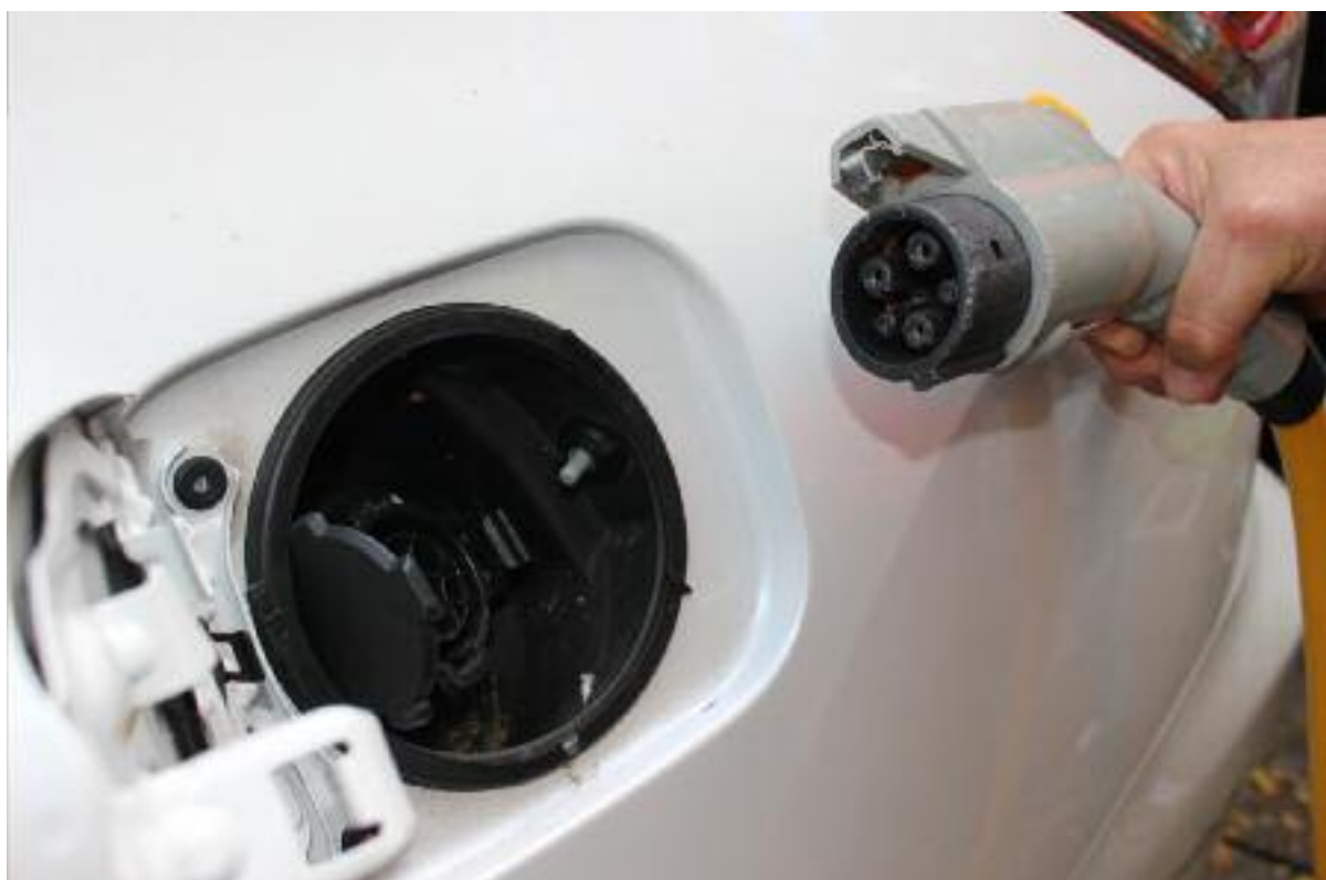
An EVSE plug to a newer electric car. Electric vehicle supply equipment provides a safer way to charge up – two prongs are for power, one for a ground, one for safety so that the power will shut off if things get gnarly, and one to communicate with the car's computer.
