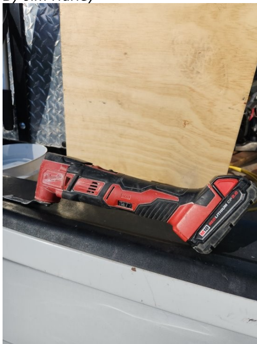
A Multi-Tool can be adapted for sanding as well as sawing. Photo Jim Hurley
